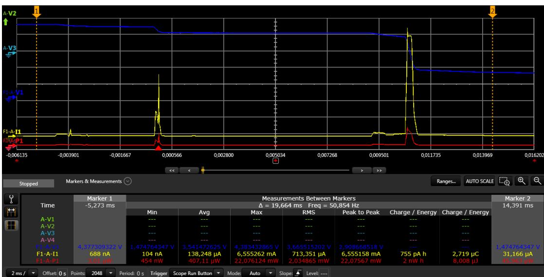
Fig. 7. 1-2 \mu F storage in system. Not enough energy for a Ble frame. The frame is wrongly transmitted (last parts truncated because there is not enough energy). But the available energy will be enough for the short frame in the proprietary system.
